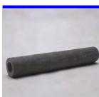
Fibre cement tube for reinforcement of waterproof walls. Acts as formwork spacer and as cover for the tie rod. In this way the thickness of the concrete walls and the reuse of the tie rods in guaranteed.
